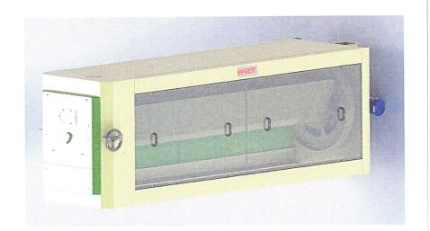
\* The MAROT indented cylinder separates grains according to length by size of the indentations in the shell. These shells are easily changed, allowing the machine to be altered to suit different lengths of grains.
